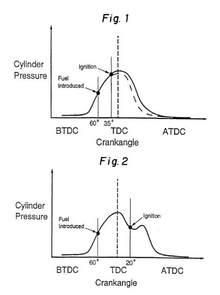
Figures 1 and 2 depict graphs showing the cylinder pressure-crankangle characteristics for a typical direct injected two-stroke internal combustion engine and for such an engine operated according to the method of the '365 patent, respectively. *Id.*, col. 2, ll. 46–52.
