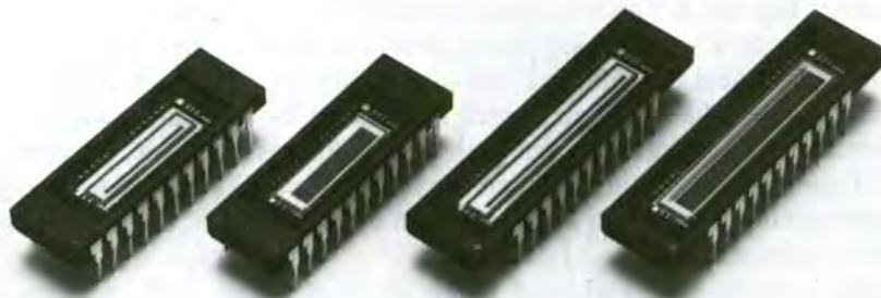
FIGURE 14.19 Photo of 1024 element diode arrays. Courtesy of Hamatsu Photonics, K. K.
