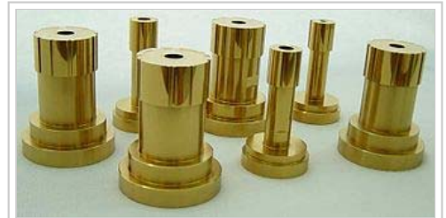
Titanium nitride (TiN) coated punches using cathodic arc deposition technique
