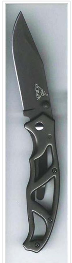
Dark gray TiCN coating on a Gerber pocketknife
