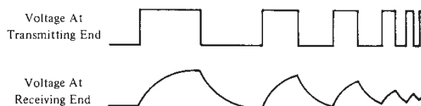
FIGURE 2.1 Attenuation of Digital Signals
