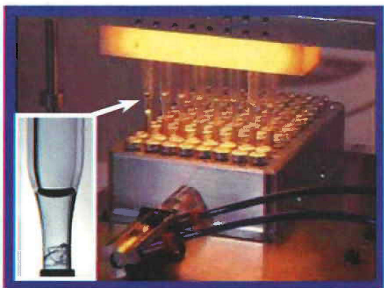
Fig. 1. Photo of optical inspection station. (Inset shows close up of crystallization vessel that contains crystals.) (Courtesy of Transform Pharmaceuticals, 2002.)
