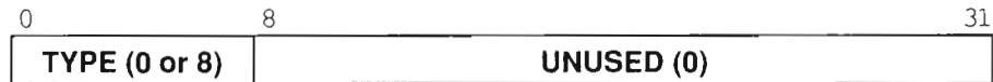
Figure 13.10 The format of a GGP echo request or reply message. Type 8 identifies the message as an echo request, while type 0 identifies the message as an echo reply.
