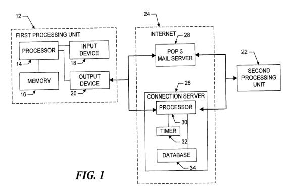
Figure 1 illustrates the architecture between first processing unit 12, second processing unit 22, and connection server 26. *Id.* at col. 5, ll. 15-29.
