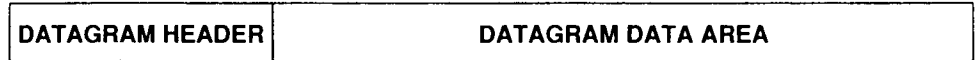
Figure 7.2 General form of an IP datagram, the TCP/IP analogy to a network frame. IP specifies the header format including the source and destination IP addresses. IP does not specify the format of the data area; it can be used to transport arbitrary data.
