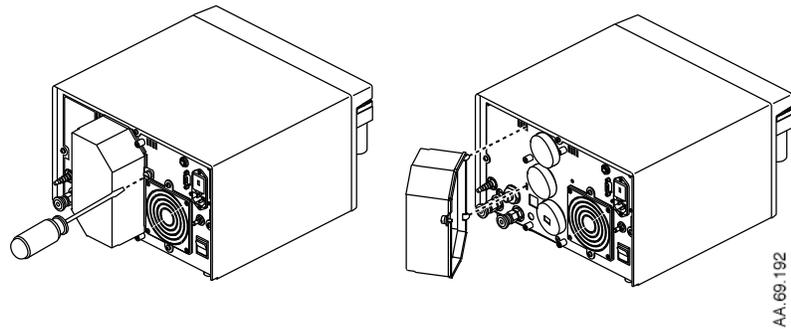
Figure 15-7 • Sensor cover removal and replacement
