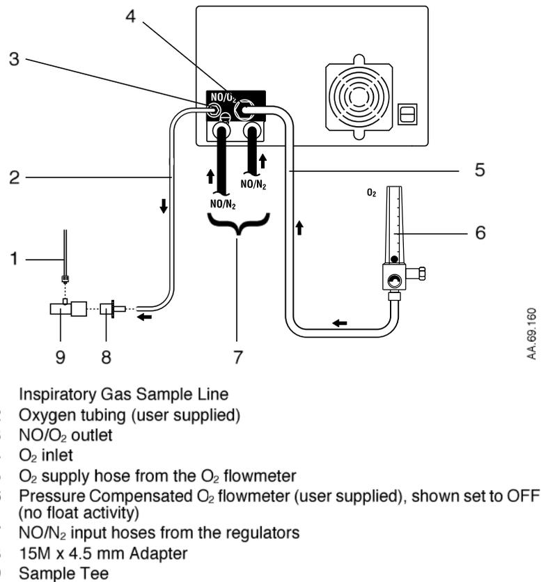
Figure 5-2 • Sample tee connection to the Manual NO delivery system
