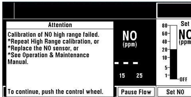
Figure 4-10 • High range calibration menu example - NO high range calibration failed
