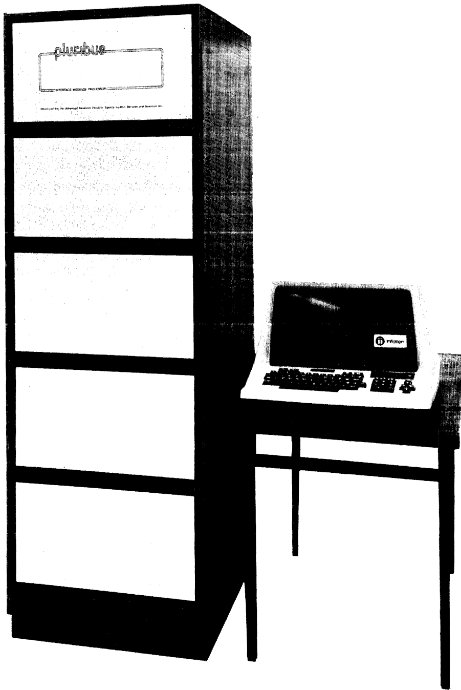
FIG. 1-5 THE PLURIBUS IMP AND IMP TERMINAL
