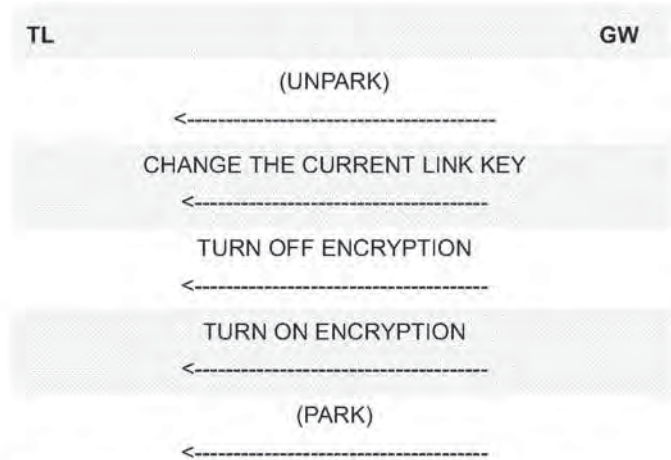
Figure 10.10: Signalling diagram for periodic key update
