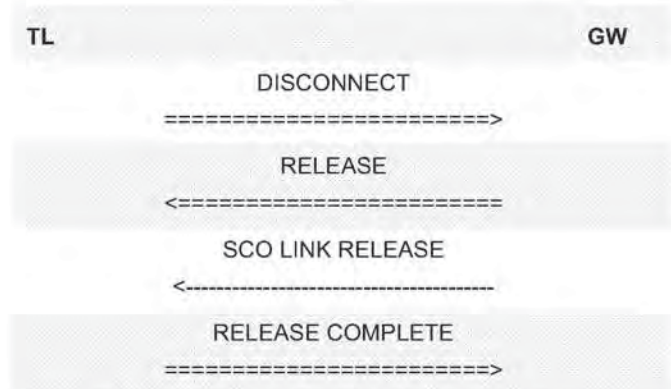
Figure 10.5: Call Clearing signalling flow, successful case
