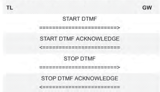
Figure 10.6: DTMF signalling, successful case
