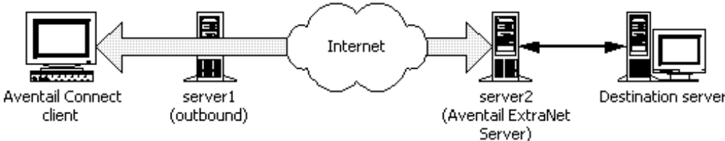
MULTIPROXY: The user authenticates with server2 directly.
