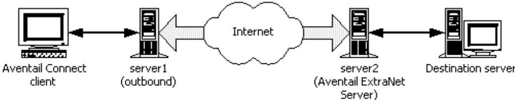
PROXY CHAINING: Server1 appears as a user to server2.
