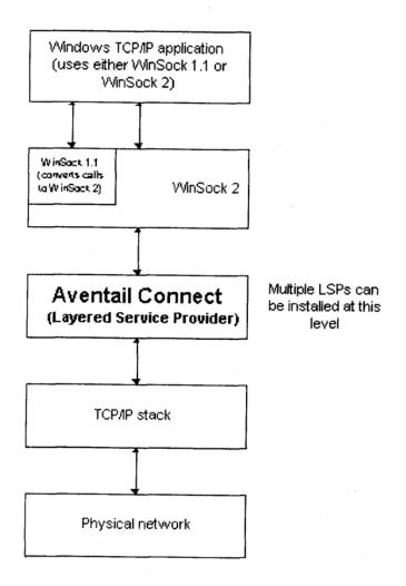
Windows TCP/IP applications and Aventail Connect have no direct contact with one another; instead, each of them communicates through WinSock. Multiple LSP applications can be installed at the LSP level.
