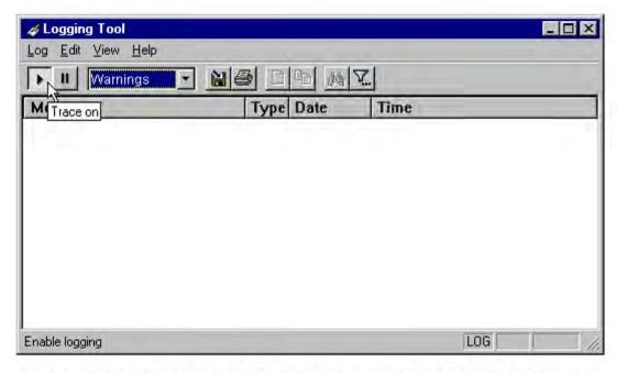
The log window will now record and display trace information as it is generated by Aventail Connect. You can tell when the trace function is active because messages are scrolling down the screen and the **Trace On** button is depressed.
