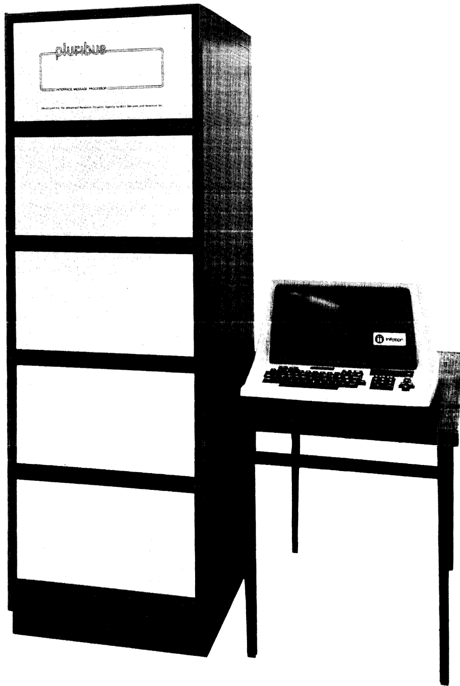
FIG. 1-5 THE PLURIBUS IMP AND IMP TERMINAL
