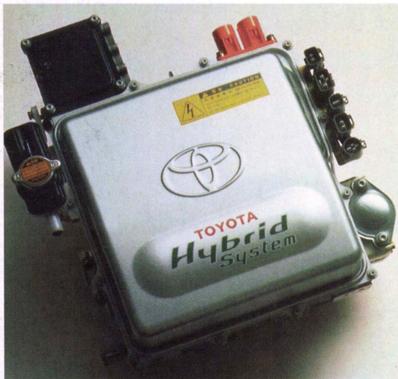
Prius' high-output nickel-hydrate battery pack (top) is positioned between the rear seat and luggage compartment. Below is the inverter unit, whose electronic elements are of Toyota's own design and manufacture, as is the motor regenerator.
