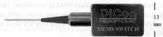
Figure 2. A simple 1x2 protection switch is one example of the optical MEMS products now commonplace in telecom systems.
