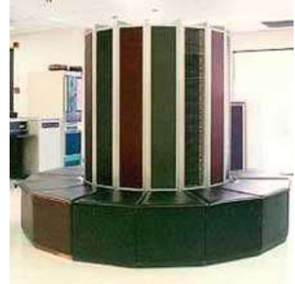
Supercomputer (this one is a Cray-2 from the 1980's)
