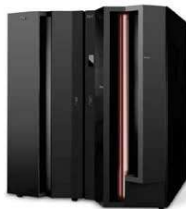
Mainframe computer (this IBM z-series computer is about 6 feet tall)
