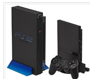
Original PlayStation 2 console (left) and slimline PlayStation 2 console with 8 MB Memory Card and DualShock 2 controller (right).
