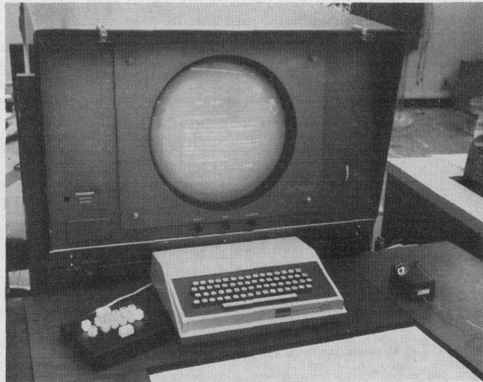
Fig. 1. The on-line system work station showing the CRT display, keyboard, pushbuttons, and mouse.
