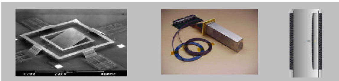
Fig.2 3D MEMS scanner, 64x64 cross connect module, 256x256 integrated solution
