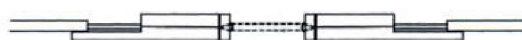
b) Schematic view of coupling optics in a pair of fiber collimator arrays.
