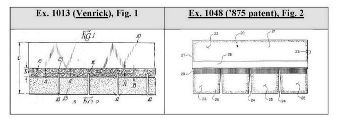
The reinforcing strip in <u>Venrick</u> can also be on the rear exterior surface of the shingle. *See* Ex. 1013 at Figs. 8–12; Ex. 1003 at ¶¶ 540, 329, 84, 87. <u>Venrick</u> states: "in Figures 8, 10, and 12 the raised median strip is located on the <u>undersurface</u> of the shingle." Ex. 1013 at 4, col. 2:60–62 (emphasis added); Ex. 1003 at ¶ 329.
