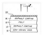
A purpose of the web layer is "<u>adding reinforcement</u>... and providing <u>additional tear strength</u>." Ex. 1014 at col. 4:17–27; Ex. 1003 at ¶ 91. The thickness of the web is on the order of 1/1000<sup>th</sup> of an inch. Ex. 1014 at col. 3:59–60 ("a thickness of between about 10 mils or less to about 30 mils"); Ex. 1003 at ¶¶ 92–93; *see also id.* at § V.B.
