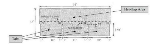
As shown, the nailing zone is (a) generally longitudinal, (b) located between the right and left edges, and (c) intermediate of the upper and lower edges. Ex. 1003 at ¶ 56.
