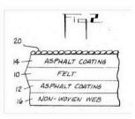
A purpose of the web layer is "<u>adding reinforcement</u>...and providing <u>additional tear strength</u>." Ex. 1014 at col. 4:17–27 (emphases added); Ex. 1003 at ¶ 91. The thickness of the web is on the order of  $1/1000^{\text{th}}$  of an inch. Ex. 1014 at col. 3:59-60 ("a thickness of between about 10 mils or less to about 30 mils"); Ex. 1003 at ¶¶ 92–93; *see also id.* at § V.B.
