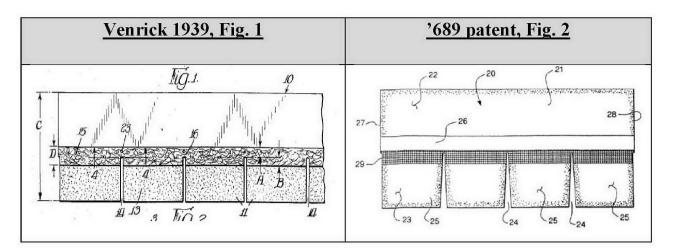
The reinforcing strip in Venrick 1939 (Ex. 1013) can be on the rear exterior surface of the shingle. *See id.* at Figs. 8–12; Ex. 1003 (Bryson Decl.), at ¶¶ 349, 629. Venrick 1939 (Ex. 1013) states: "in Figures 8, 10, and 12 the raised median strip is located on the *undersurface* of the shingle." *Id.* at 4, col. 2:60–62 (emphasis added); Ex. 1003 (Bryson Decl.), at ¶¶ 349, 629.
