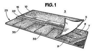
The shingle comprises an upper layer 5 and a lower layer 7, which are glued together with a sealant 9. Ex. 1003 (Bryson Decl.), at  $\P$  72. The upper layer includes a headlap area 10 and a number of tabs 35. *Id*. The lower layer is longitudinal, and extends between the right and left edges. *Id*.
