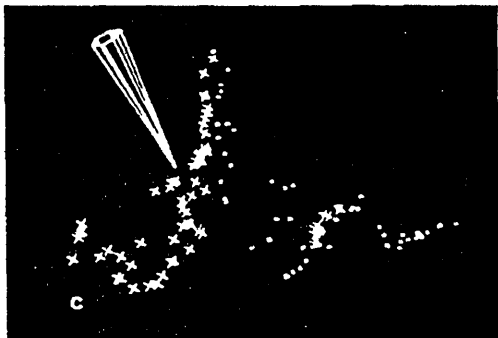
Fig 5 To collect a 3 D point the surgeon positions the pointer tip in contact with the vertebral surface and presses a foot pedal (a) Acquisition during in vitro experiments (b) Acquisition during actual surgery (c) The result is a set of 3 D surface points lying on the vertebral surface. Motions of the vertebra are compensated through an internal coordinate system fixed to the spinous process
