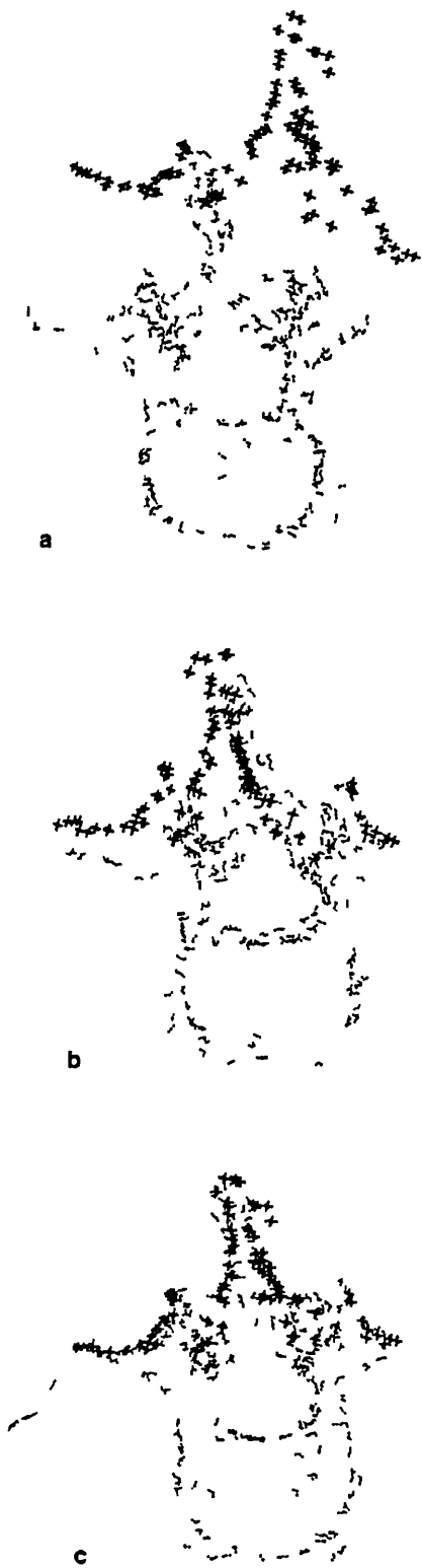
Fig 6 Iterative registration of 3 D data points with the surface model segmented in CT images (a) Initial position (b) Intermediate position (c) Final position The convergence is reached in about 2 sec on a DEC5000
