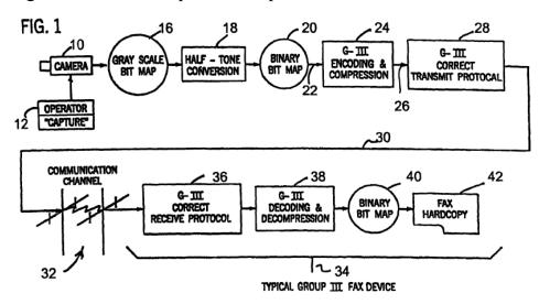
Figure 1 is a block diagram of a basic facsimile camera configuration for capturing an image via a camera and transmitting it via Group III facsimile transmission to a standard hard copy medium. *Id.* at 4:27–30.
