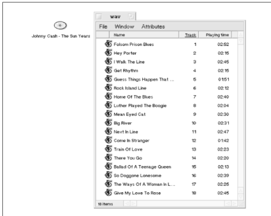
Figure 5.5. Tracks on audio CDs in BeOS appear to the Tracker as WAV files
