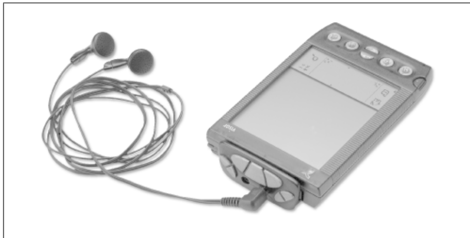
Figure 6.9. The InnoGear MiniJam is an expansion module for the HandSpring Visor PDA
