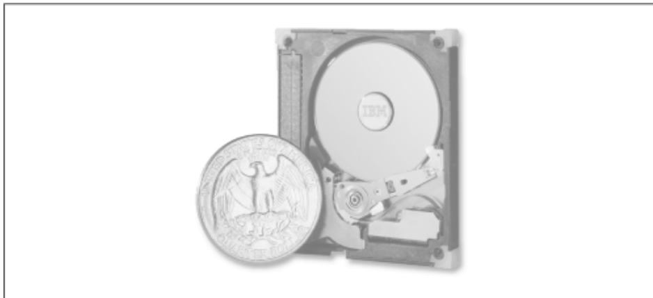
Figure 6.4. IBM's MicroDrive stores 340 MB of data and is small enough to be used in portable MP3 devices
