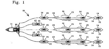
Ex. C, DX 266 at 2 (emphasis added); *see also id.* at 6 (col. 3, ll. 14-21) ("streamer positioning devices 14, for example birds and tail buoys, may be attached to the exterior of the streamer cables 13 for adjusting the vertical and lateral positions of the streamer cables 13."); *see also* Ex. A, Tr. at 3829:19 – 3830:7.
