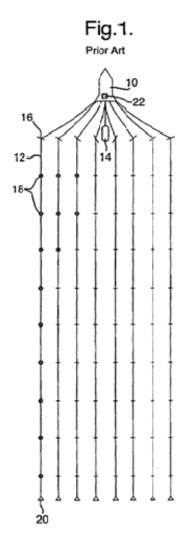
Figure 1 depicts an array of seismic streamers 12 towed behind the vessel.
