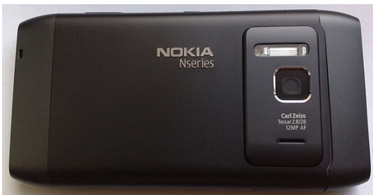
The Nokia N8 smartphone is the first Nokia smartphone with a 12-megapixel autofocus lens, and is one of the few camera phones (the first was Nokia N82) to feature Carl Zeiss optics with xenon flash.
