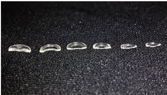
Image showing the six molded elements in the Samsung Galaxy S5
