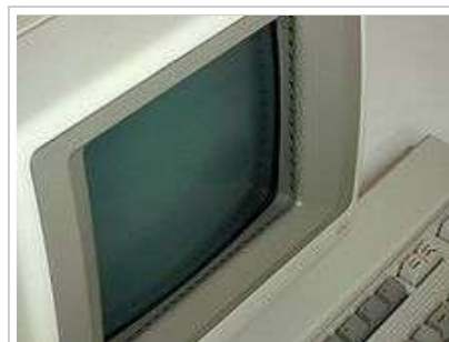
HP Series 100 HP-150 c. 1983, the earliest commercial touchscreen computer
