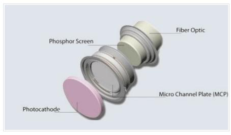
Channel Plate (MCP). An MCP Visualisation of image intensifier with Micro Channel Plate
