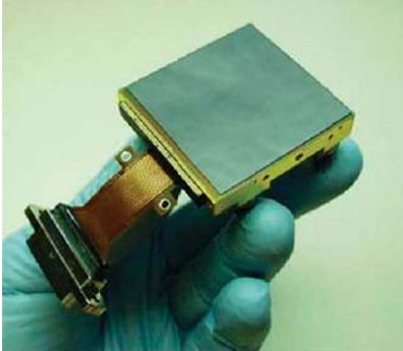
FIGURE 2. The HAWAII-2RG (H2RG) is a 2048 \times 2048 -pixel imaging array. (Courtesy of Teledyne Imaging Sensors) Click here to enlarge image
