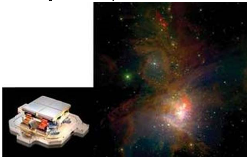
FIGURE 1. The Orion Nebula was imaged with the WIRCam (Wide Field Infrared Camera) of the 3.6 m Canada-France-Hawaii Telescope in Hawaii. WIRCam is based on a 4096 \times 4096 -pixel mosaic of four H2RG short-wave (1 to 2.5 \mu\text{m} ) sensors (inset). Most of the red stars in this image were first observed with the advent of IR cameras. (Courtesy of Canada-France-Hawaii Telescope)
