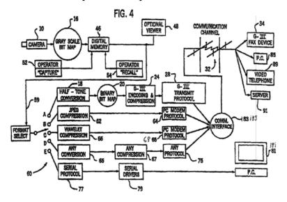
Figure 4 of the '168 Patent illustrates the data path after an image is captured by camera 10 and conditioned by gray scale bit map 16. *Id.* at 7:65–8:41. The device includes memory 46, optional viewer 48, and format select
