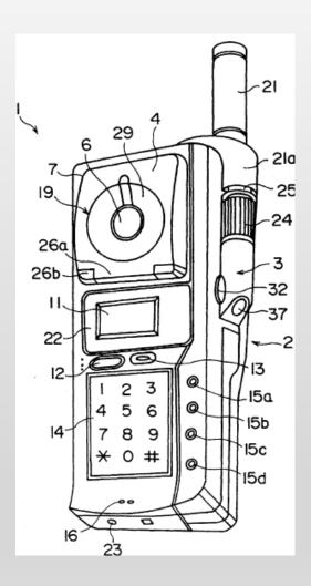
FIG. **1** shows a perspective external view of embodiment of a video telephone according Umezawa.
