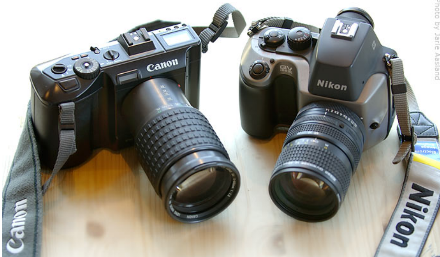
Canon RC-760 with a 11-66mm f/1.2 and Nikon's first still video camera, the extremely rare QV-1000C. The Nikon lens is a special 10-40 mm f/1.4 QV Nikkor. Unlike its competition, Nikon's first filmless camera would only capture grayscale (black and white) images. And -- it was also much more expensive than the Canon models.
