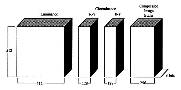
The framestore board, which has a total capacity of 512 kbytes, includes memory space for the compressed image data. The original uncompressed image occupies 384 kbytes of memory, therefore 128 kbytes are available to be used as the compressed image buffer.
