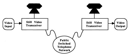
The input to the system can be any source of NTSC composite or RGB video in still or motion form. The output from the system can be connected to any device that accepts NTSC composite or RGB video.
