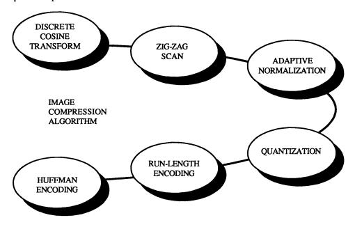
The results of the transform, which are coefficients representing the spatial energy within the block, are then scanned into a one-dimensional array so that the first term represents the lowest spatial frequency and the last term represents the highest spatial frequency.
