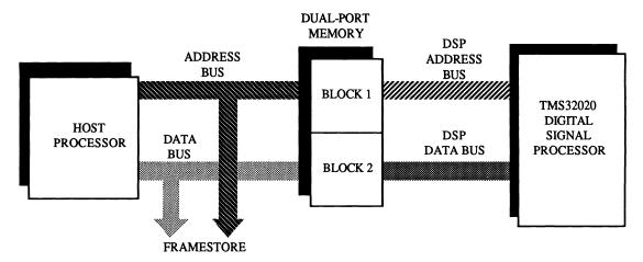
This switching back and forth is repeated until the entire image is processed. A single memory location is defined for each block as the communication link between the two processors. Writing to its location allows the microprocessor to instruct the DSP as to which operation should be performed, and the DSP notifies the microprocessor it has completed its processing on the block by writing to its location.
