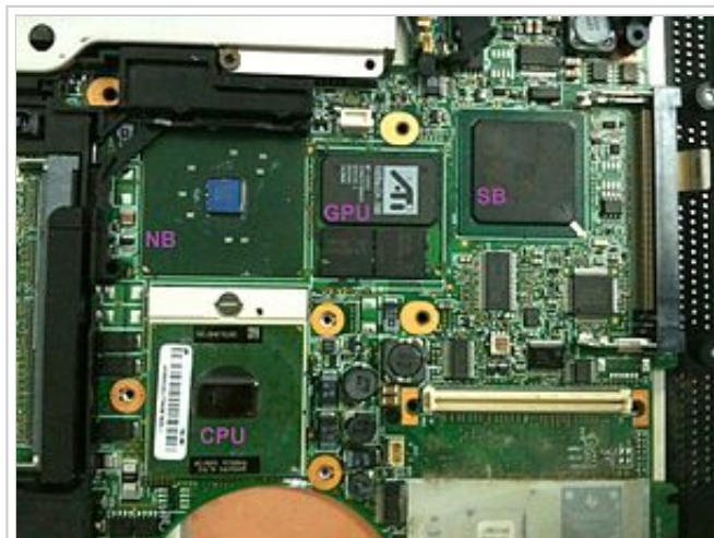
A part of an IBM T42 laptop motherboard. CPU: Central processing unit. NB: Northbridge. GPU: Graphics processing unit. SB: Southbridge.
