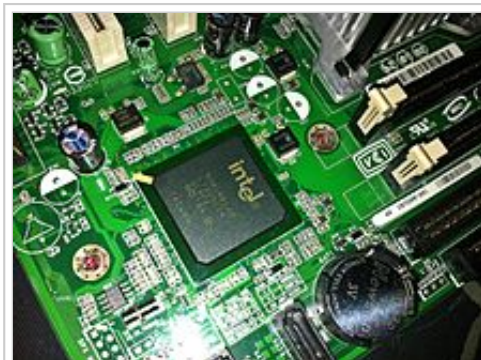
Intel ICH7 Southbridge on Intel D945GCPE Desktop Board
