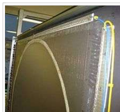
Back side of a Multitouch Globe, based on Projected Capacitive Touch (PCT) technology
