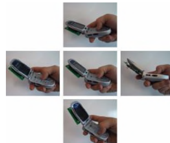
Figure 1. TiltText . The center picture shows the untilted phone where pressing a key enters its numeric value. Left picture: left tilt enters first character on key. Top picture: forward tilt enters second character. Right picture: right tilt enters third character. Bottom picture: tilting towards the user enters fourth character if one exists for that key.
