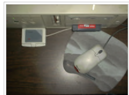
A Cirque Easy Cat Desktop touchpad compared with a mouse and mousepad.
