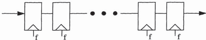
Figure 9a: Shift Register without Parallellization
