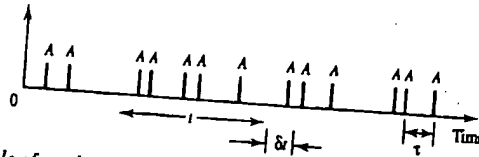
Figure 17.3 Example of randomly distributed arrivals (A) with interarrival time \tau . Only arrivals then the probability of being in state j after \delta t seconds is dependent on P_j and P_{j-1} :
