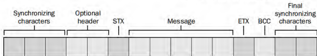
BISYNC. The structure of a BISYNC frame.
