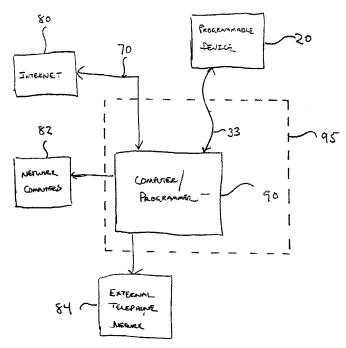
(57) Abstract: A device for programming user-defined information into an electronic device is provided. The programmer allows a user to program customized information, such as user-selected audio, video, or Internet access information into his or her programmable device. Such electronic devices include wireless telephones, pagers, and personal digital assistants. The programmer allows a user to, among other things, customize the device to suit his or her particular taste.
