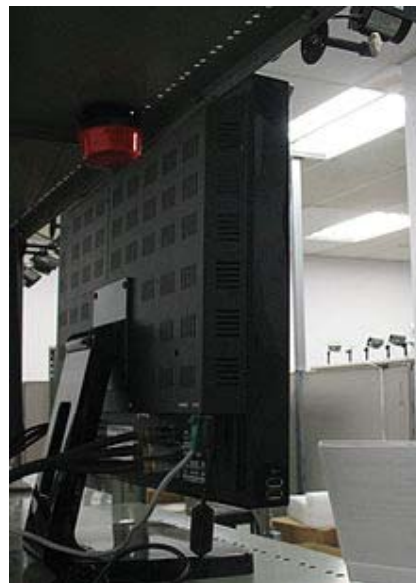
Side view: Even with all the DVR components inside, the LCD monitor is still slim.
