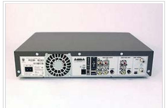
Back view of a TiVo Series2 5xx-generation unit.
