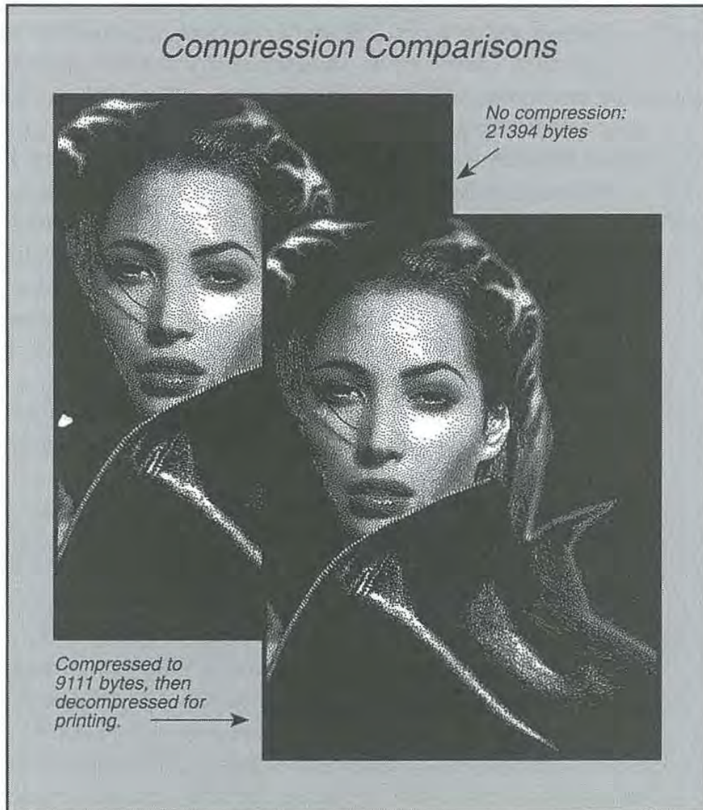
Figure 5-15: The original image on the left measures 21,394 bytes. The image on the right was compressed to 9,111 bytes (43 percent of the original), then decompressed for printing. No data was lost; both pictures are identical. (Graphic enhancement by David Palermo using Adobe PhotoShop.)
