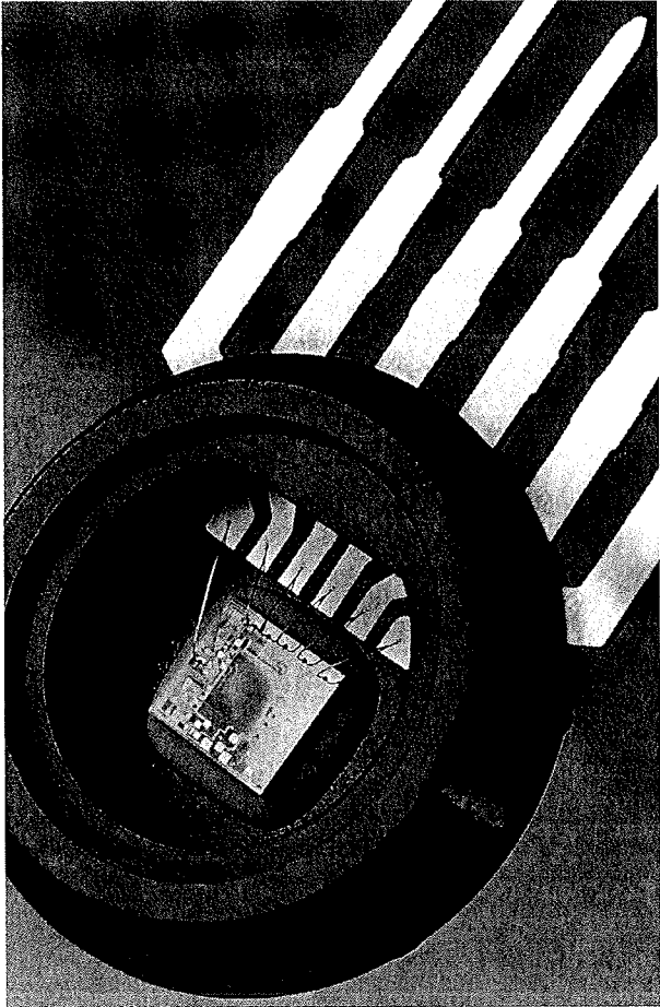
FIGURE 2.8 Silicon pressure sensor with integrated electronics. (Courtesy Motorola, Inc.)
