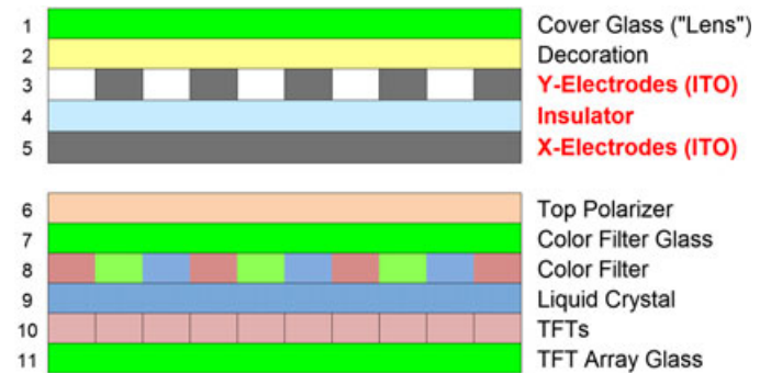
FIGURE 5 — This figure depicts the p-cap “one-glass solution” (also called “sensor on lens”) configuration used by the touchscreen industry. To eliminate the fourth piece of glass, the p-cap electrodes are moved to the bottom surface of the decorated cover glass (rows 3–5). ITO, indium tin oxide; TFT, thin film transistor. Source: the author.
