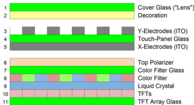
FIGURE 4 — All smartphones and tablets use some form of “decorated covering” (rows 1 and 2) to protect the LCD (rows 6–11) from damage. When a projected capacitive touchscreen is added, most commonly, the electrodes are located on a fourth piece of glass (rows 3–5). ITO, indium tin oxide; TFT, thin film transistor. Source: the author.
